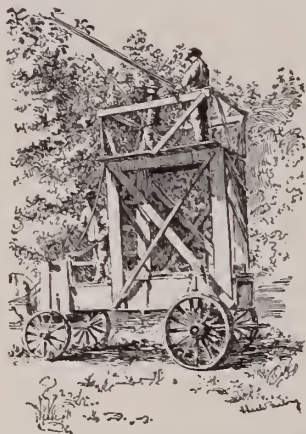
2377. Square tower, giving more working space for the nozzle-men than the conical form.
